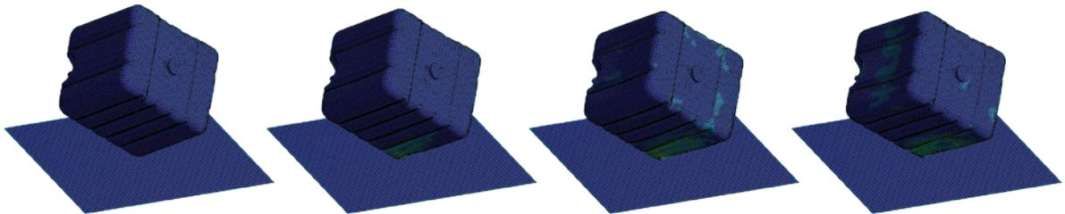
Equivalent stress buildup during drop testing from height of 1 meter
